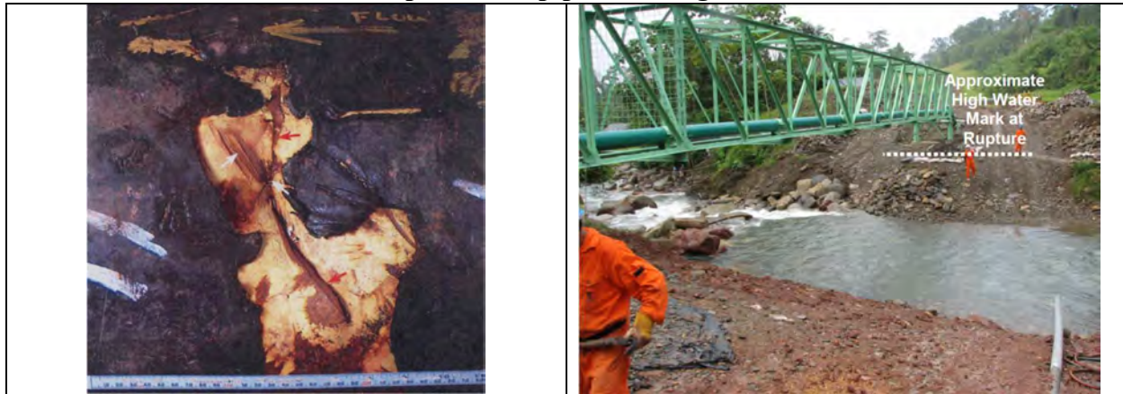
Figure 10. Photographs of the open-cut buried pipe section that ruptured and the replacement pipeline bridge 110
